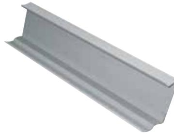
CasoLine quick-lock GRID Main Tee CLT15P sections are cut to suit the width of the corridor. The section length should be no more than 10mm shorter than the corridor width. Main Tee sections are fitted into the CasoLine quick-lock GRID Shadowline Moulding CLSM04, onto the upper recessed flange. There is no requirement to install hangers to support the CasoLine quick-lock GRID Main Tee sections. These sections should not be joined and no soffit supports or hangers are required.
