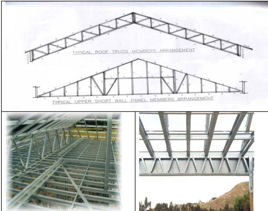
Figure 9.17 Roof Truss
